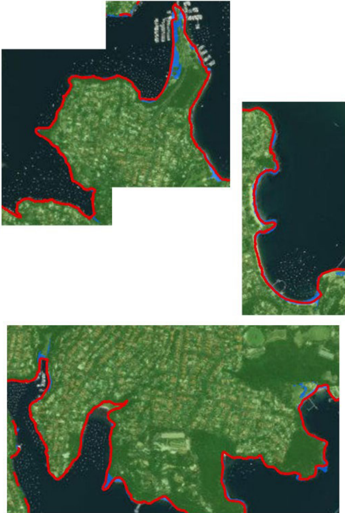
Figure 13: Enlarged map of projected coastal inundation for Mosman by 2100, based on RCP 8.5 and 0.78 m sea level rise. Source: CoastAdapt
